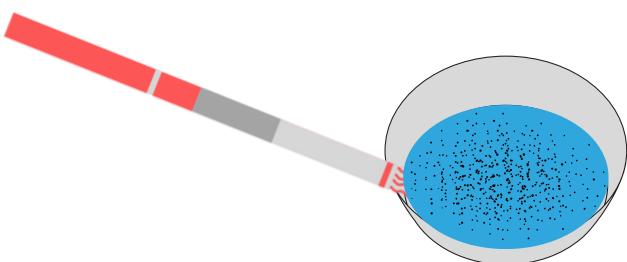
**4** Remove the strip and lay it on a clean, flat surface. Wait 2-5 minutes for the results.
